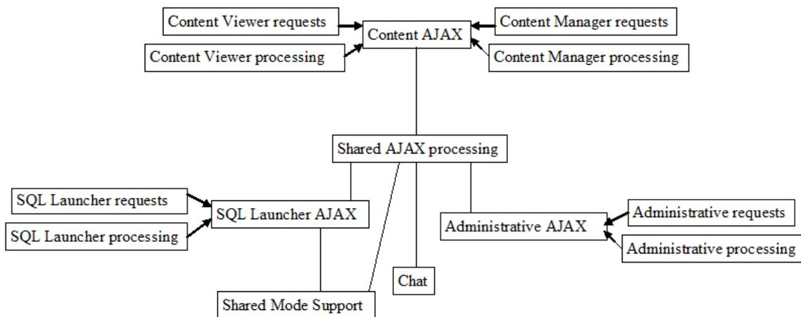
**The basic functional structure of the AEQ tool AJAX client (note that Shared Mode Support borrows functionality from SQL Launcher as well as shared functions)**
